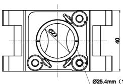
Ø25.4mm (1 in.) optics secured by retaining with recommended Thickness: 1 to 4mm
